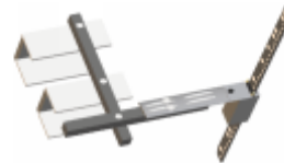
Figure 10: Sensor Mounting Plate Crosshead Installation
