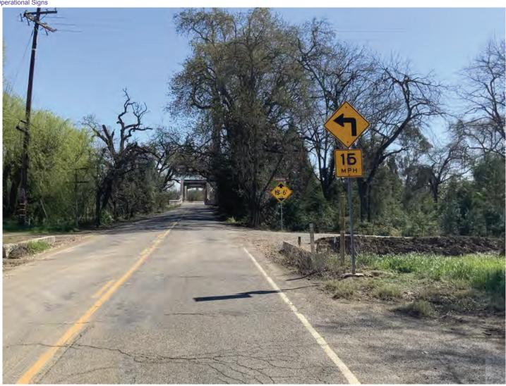
Photo #7 Vertical clearance 13 FT 6 IN and 15 MPH signs at the approach to Abutment 5.
