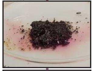
**Figure 1:** Pure iodine crystals, heated slightly, showing some solid iodine escaping directly to the air as obvious violet-colored vapors. Because of this "sublimation" property, exposures include dermal contact with solid crystals and inhalation of vapors which may not be quite as visible as this at room temperature. *Photographer, Charles Salocks.*
