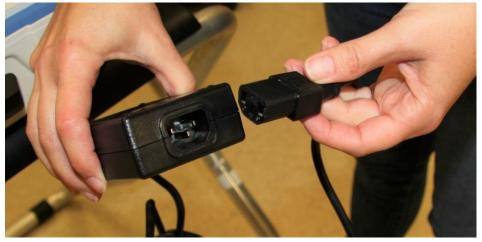
Unplug the power cord from the back of the Touch Writer. **Note that there is a locking sleeve that must be pulled back from plug on back of Touch Writer!** To disconnect the power cord, grasp the cord at the base of the black connector molding and slide back the sleeve. This will unlock the connection so that the cord can be removed.
