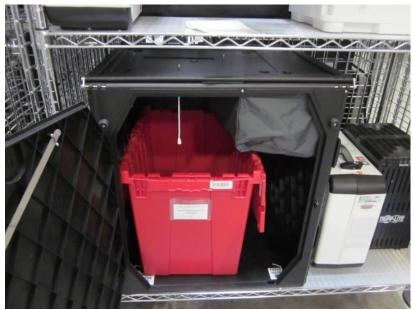
Remove ballot scanner from caddy and place on ballot box. Place feet on bottom of scanner into indentations on top of ballot box.
