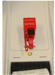
Plug the Touch Writer power cord into a wall outlet. A green light will illuminate on the power brick when AC power is present
