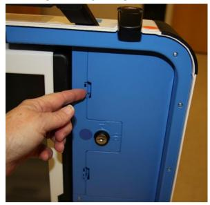
Remove power brick and cord from storage compartment, replace storage compartment cover, then close lid of scanner.
