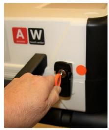
Reaching under the Touch Writer table, pull the metal latch toward you to unlock the Touch Writer from the booth.
