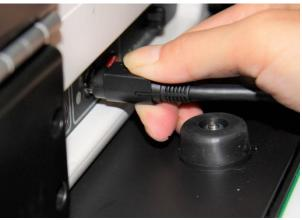
Remove blue cover from power cord storage compartment, and neatly place cords back inside. Replace blue cover.
