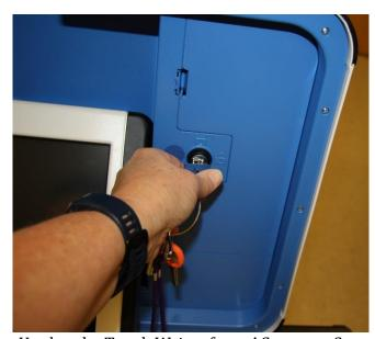
Unplug the Touch Writer from AC power. Separate the power cord from the power brick.
