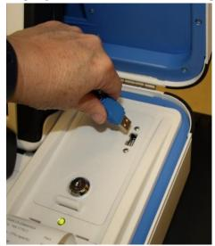
Unplug the laser printer from the back of the Touch Writer.
