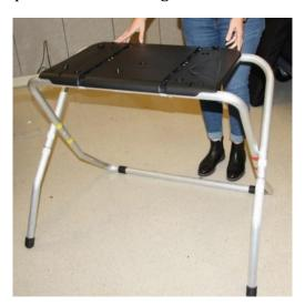
Set up the Touch Writer table and Touch Writer near the caddy with the UPS inside. Place the Touch Writer on the table, lining up the feet with the indentations on the table, and lock into place with metal tab under table; push tab to back of table to lock Touch Writer in place. Pull up on Touch Writer to check that it is locked onto the table.
