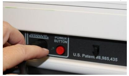
When the Ballot Scanner is completely powered down and is displaying a black screen, unlock the tablet using the blue key.
