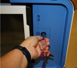
Seat the tablet firmly in the cradle with two hands, tilt back, and using the blue key, lock it in place.
