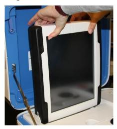
Stow the tablet in the storage area in the case cover, move the latch to hold the tablet, then lock the tablet in place with the blue key.
