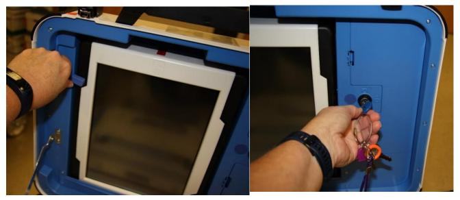
Seat the tablet firmly in the cradle with two hands, tilt back, and using the blue key, lock it in place.
