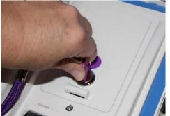
Remove the vDrive by pulling it straight up and out. Replace vDrive door.
