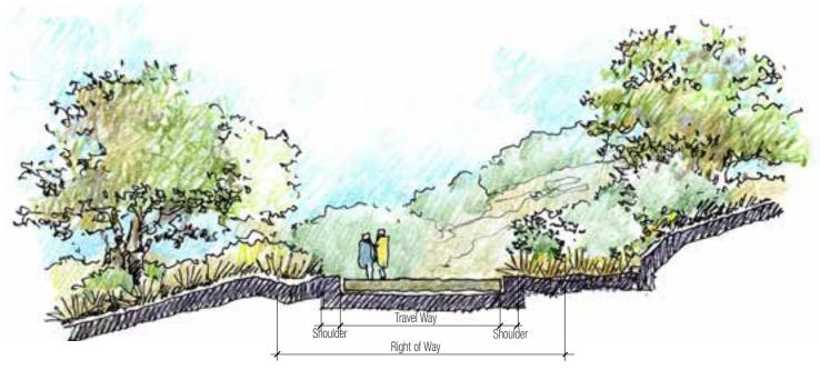
Figure 5-80: Emergency Access/Fire Road Section
