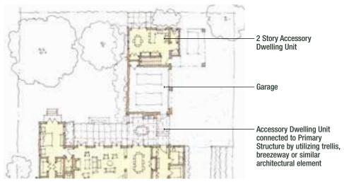
Figure 5-39: Conceptual Secondary Unit Plan Sketch
