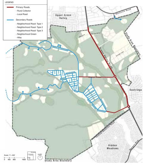
Figure 5-66: Primary and Secondary Thoroughfares
