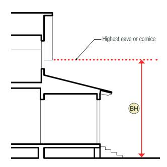
Figure 5-35: Compound - Building Height Diagram
