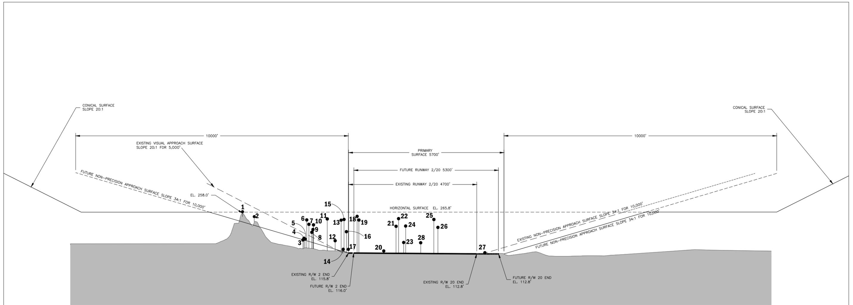
NOTE: TERRAIN PROFILE REPRESENTS THE HIGHEST POINT ACROSS THE WIDTH AND ALONG THE LENGTH OF THE APPROACH SURFACE.
