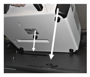
Reach inside ballot box and pull cord away from you to lock the lid and ballot scanner into place. Pull up on scanner handle to confirm scanner is locked on the ballot box.
