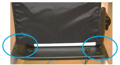
Plug the UPS on the caddy into AC power. The UPS is located on the bottom shelf of the caddy and the plug will be accessible on the back of the caddy. Do not plug the UPS into a power strip. It must be plugged directly into the wall.
