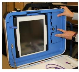
Plug power cord into brick, then plug power connector into back of ballot scanner, flat side up. You will hear a soft click when inserting the plug into the back of the
