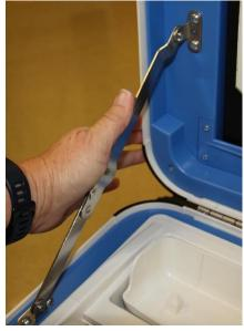
Unlock (blue key), unlatch and remove tablet
