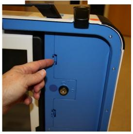
Remove power brick and cord from storage compartment from ballot scanner case, replace storage compartment cover, then close lid of scanner.
