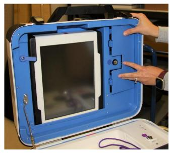
Plug power cord into brick, then plug power connector into back of Touch Writer, flat side up. You will hear and feel a soft click when inserting the plug into the back of the Touch Writer. Do not plug the Touch Writer into the wall yet.
