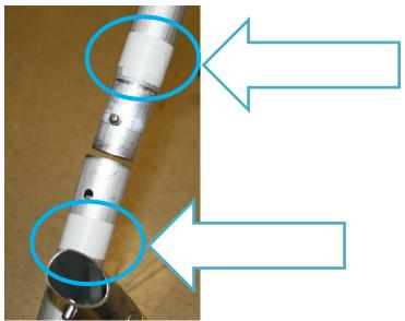
Insert "U" shaped table leg, red tape to red tape and yellow tape to yellow tape.
