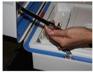
Using key with orange cover, lock case.
