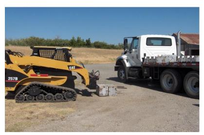
Testing of these scales is very labor intensive and requires specialized equipment. Shown here (left), is the Division's heavy weight truck and a tracked BobCat used to transfer the 500 pound certified test standards from the truck to the scale. The BobCat is extremely useful in maneuvering around corrals, through gates, and up ramps to the scale deck. A hand cart is then used to maneuver the standards around on the scale deck.
