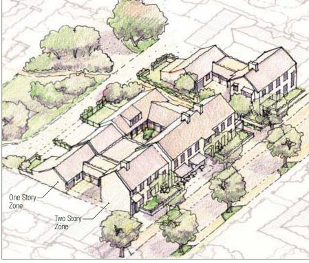
Figure 5-11: Massing Diagram: Simple Barn or Winery Forms
