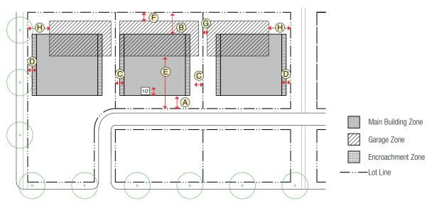
Figure 5-23: Building Placement Diagram
