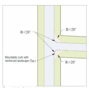
Figure 3-26: Curb design utilizing tight curb radii reduces pavement and calms traffic
