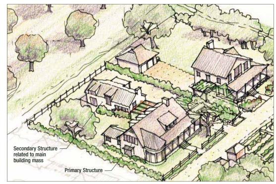
Figure 5-37: Massing Diagram
