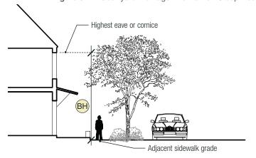
Figure 5-13: Courtyard - Building Height Diagram
