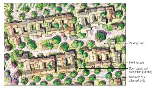
Figure 5-10: Courtyard Conceptual Layout Plan
