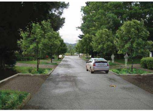
**Figure 3-14:** Roads and Streets Sustainable Design Approach - By utilizing a more efficient site design, the space can be used for stormwater infiltration and additional landscaping to encourage slower vehicle speeds and increase pedestrian safety.
