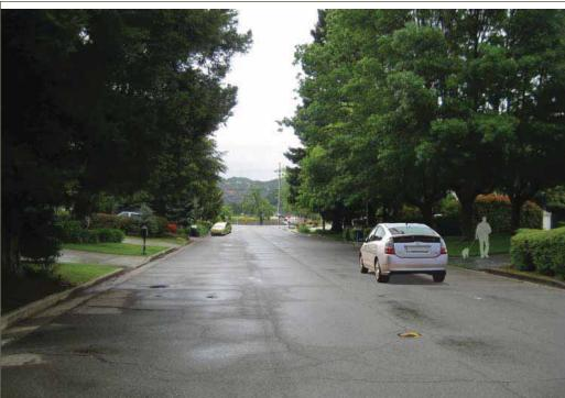
Figure 3-13: Roads and Streets Typical Design Approach - This suburban street is almost 100% impervious and designed primarily for auto flow. This combination contributes to higher auto speeds and large quantities of stormwater runooff.
