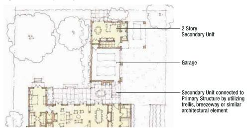
Figure 5-39: Conceptual Secondary Unit Plan Sketch
