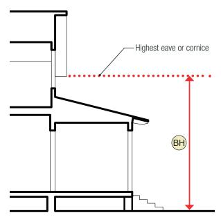
Figure 5-35: Compound - Building Height Diagram
