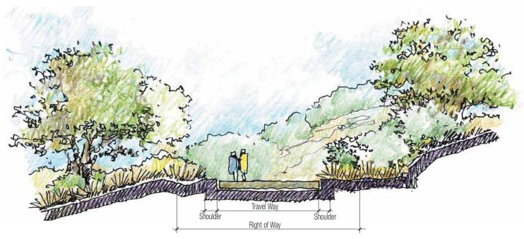
Figure 5-80: Emergency Access/Fire Road Section
