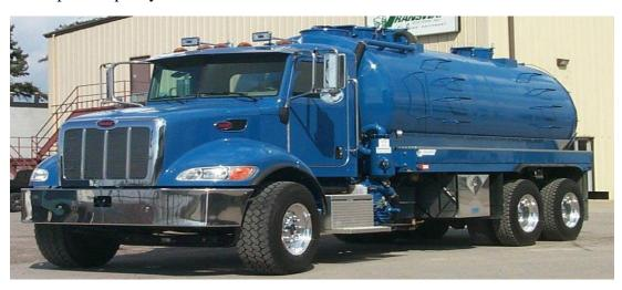
Example of typical type of pumper truck used to transport liquid waste
